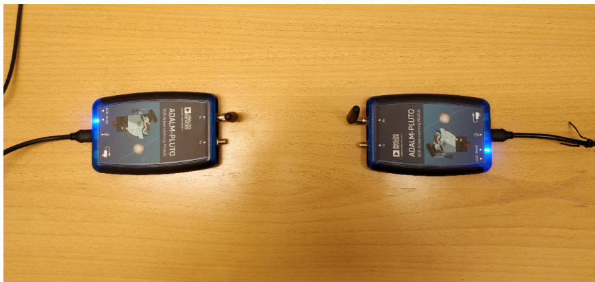
Figure 1: The figure shows the hardware used for the project, two Pluto SDR devices.
