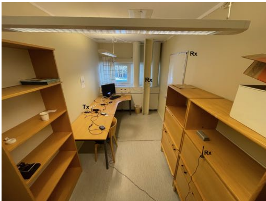
Figure 1: The antenna setup used in the tests. The transmitter (Tx) and the three receivers (Rx) are marked in the picture.
