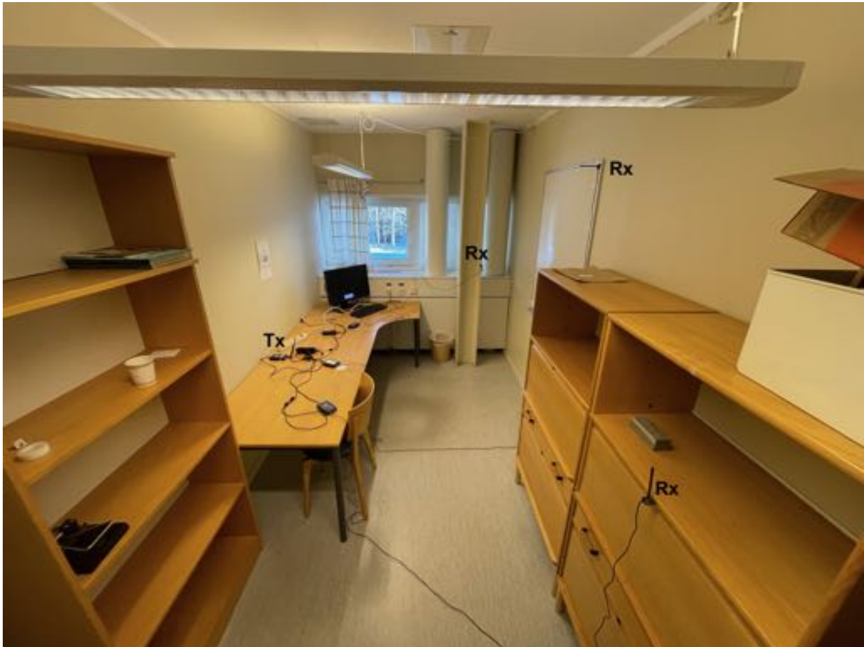
Figure 3: An example of an environment using extra long cables for better antenna placement.
